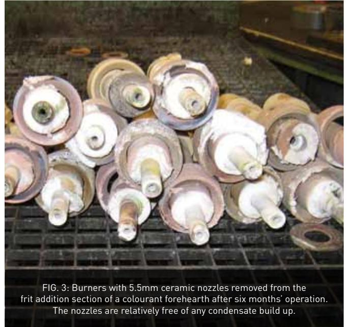
FIG 3: Burners with 5.5mm ceramic nozzles removed from the frit addition section of a colourant forehearth after six months' operation. The nozzles are relatively free of any condensate build up.
