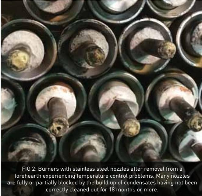
FIG 2: Burners with stainless steel nozzles after removal from a forehearth experiencing temperature control problems. Many nozzles are fully or partially blocked by the build up of condensates having not been correctly cleaned out for 18 months or more.
