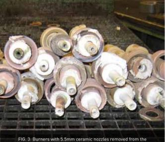
FIG. 3: Burners with 5.5mm ceramic nozzles removed from the frit addition section of a colourant forehearth after six months' operation. The nozzles are relatively free of any condensate build up.
