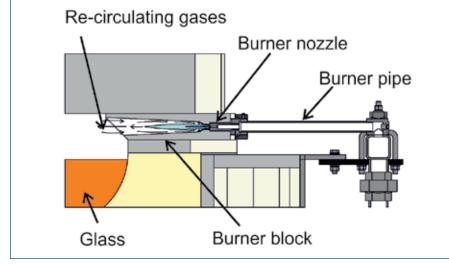
FIG 1: Forehearth Burner And Refractory Burner Block Assembly.
