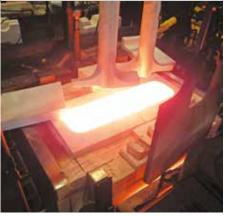
addle type stirrers being installed in a PSR CI
