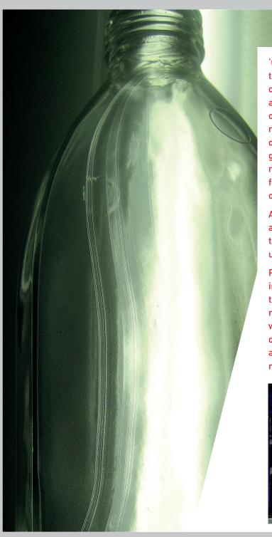
'Cat Scratch' cord is a defect in glass tableware and containers comprising a line or series of lines on the surface of the glass article. It originates from the exudation of glassy phase material in fusion cast AZS refractories used in the furnace. Being denser and more viscous than the base glass, this alumina and/or zirconia enriched material settles out on the bottom of the forehearth and is drawn onto the surface of the glass product.
