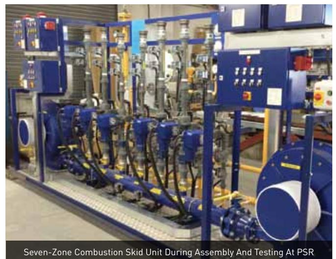
Seven-Zone Combustion Skid Unit During Assembly And Testing At PSR
